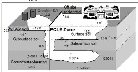
Figure 10. PCLE zone determination (mg/kg and mg/L)...
