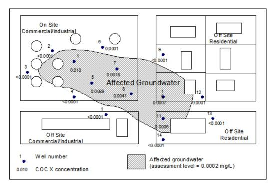
Figure 9. Horizontal Delineation of COC X in Groundwater.
