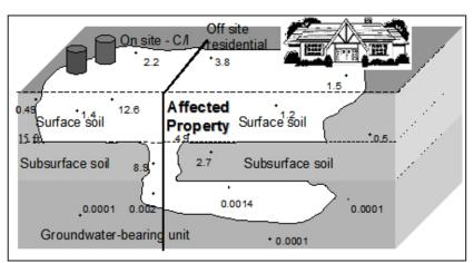
Figure 7. Affected Property Determination (mg/kg and mg/L)...
